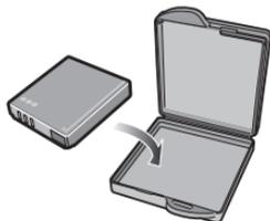
**If you drop the battery accidentally, check to see if the battery body and terminals are damaged.**
